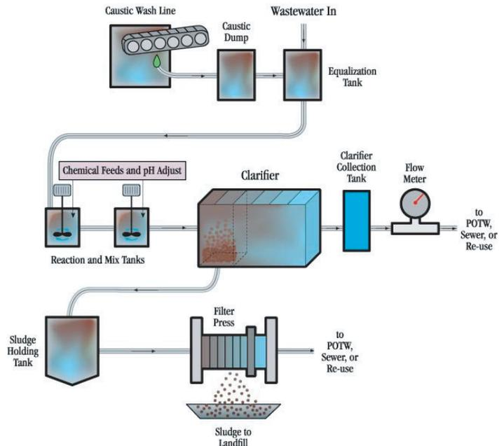
*Evergreen's polyethylene recycling processes essentially give rise to two separate waste streams: one containing all rinse water and which is held in an equalization tank, and a second stream containing highly caustic water which is collected in a caustic dump tank. Beckart engineers programmed the system to slowly meter the caustic stream to the EQ tank, which allows the water to balance out before proceeding through the treatment cycle.*
