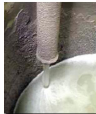
*Clear, treated water arrives in the filtrate tank, where it is subsequently routed to a larger filtrate holding tank for reuse or to the sewer.*
